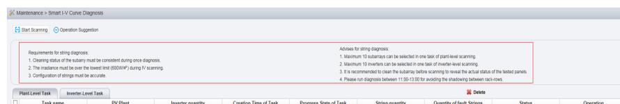
The content in the red frame in [Figure 5-25](#) is the conditions and suggestions for smart I-V curve diagnosis. Read the content carefully and ensure that the conditions are met. To minimize the content, click **Operation Suggestion**.
