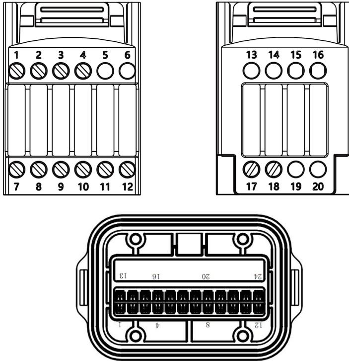
Note: 1) Pin11 is the power supply+12V, and Pin10 is the corresponding GND used;
