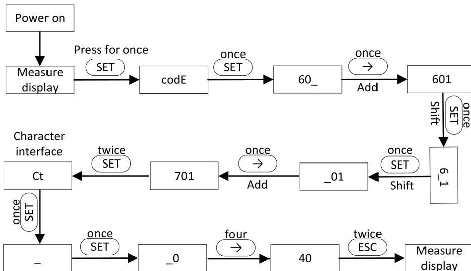
Schematic diagram of H3-Pro system 0 grid connection:
