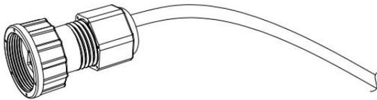
Step 3: Crimp the cable with a Rj45 plug which is inside of the cable connector.
