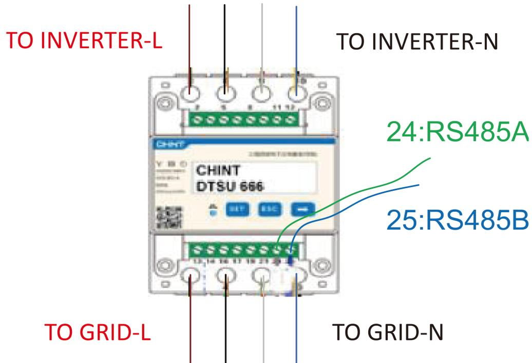
Insert L1/L2/L3/N wires and RS485A/B cable into the meter. Please refer to the meter wiring diagram on side of meter itself.
