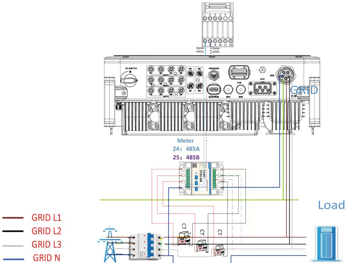
Insert L1/L2/L3/N wires ,CT and RS485A/B cable into the meter.Please refer to the meter wiring diagram on side of meter itself.
