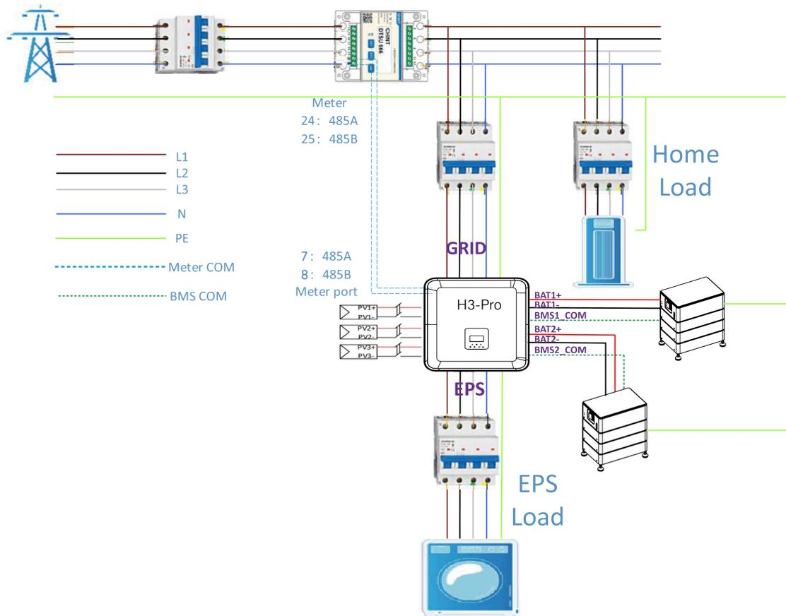
Important: H3-Pro needs to be connected to the 3-phase 5-wire power grid system, and ensure that the GRID is connected to the N line, otherwise the machine will report the SW BUS VOLT fault.
