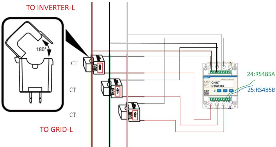
Notes: The 2,5,8 of the CT meter are connected to the three live wires L1, L2, and L3 respectively.
