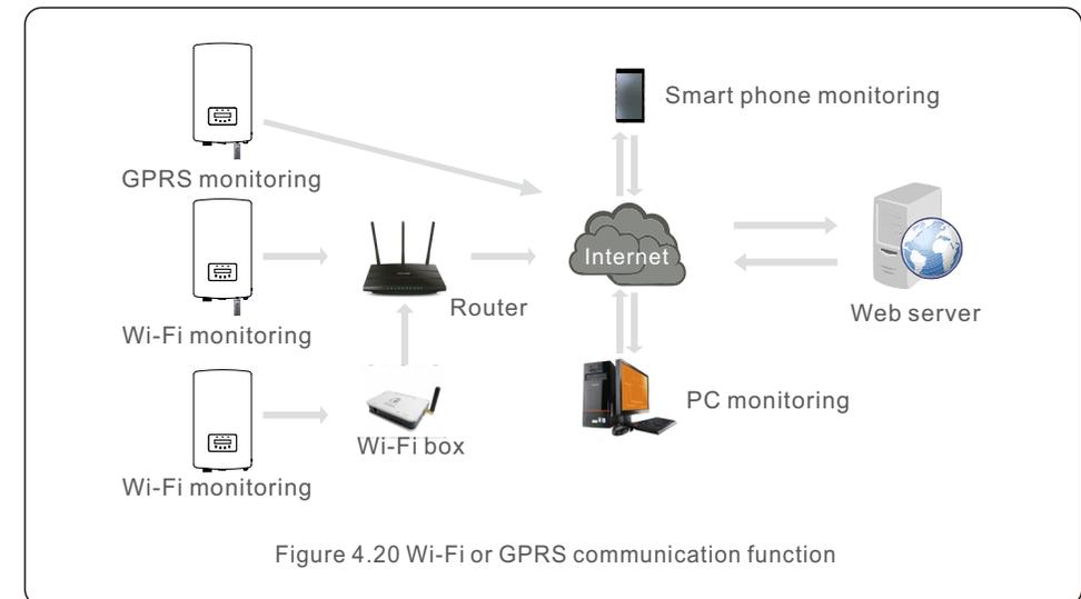
Figure 4.20 Wi-Fi or GPRS communication function
