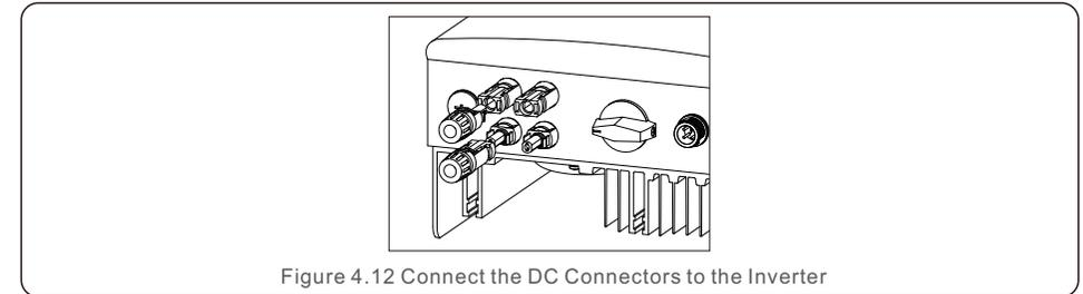
Figure 4.12 Connect the DC Connectors to the Inverter
