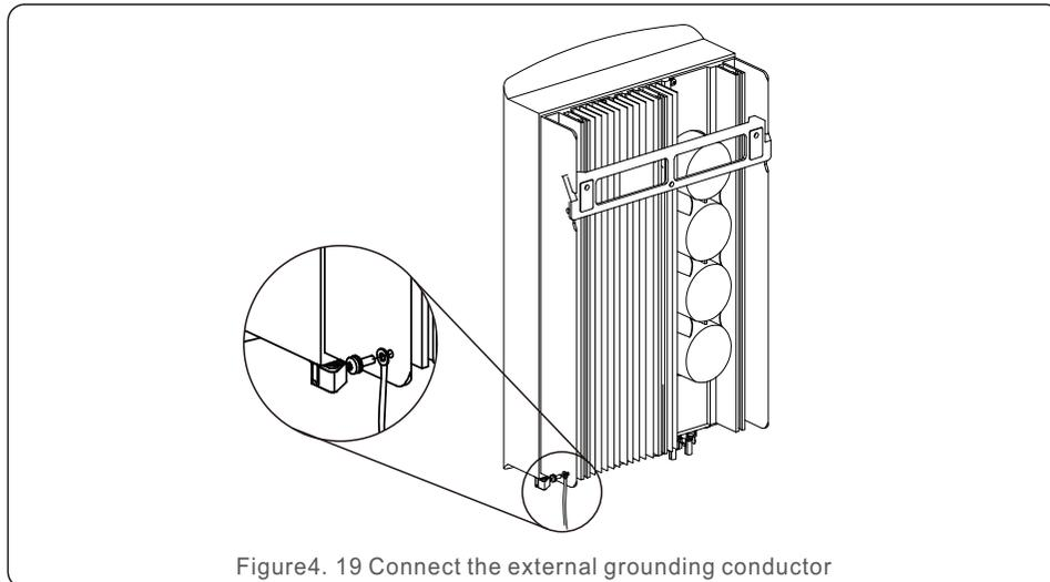
Figure4. 19 Connect the external grounding conductor
