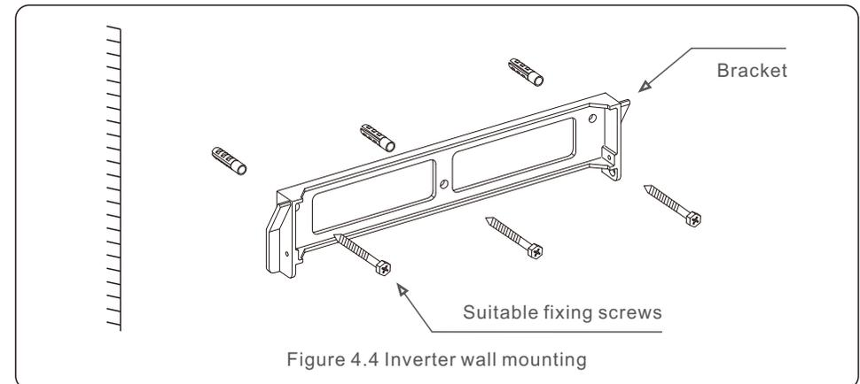
2. Make sure the bracket is horizontal. And the mounting holes (in Figure 4.4) are marked correctly. Drill the holes into wall at your marks.
