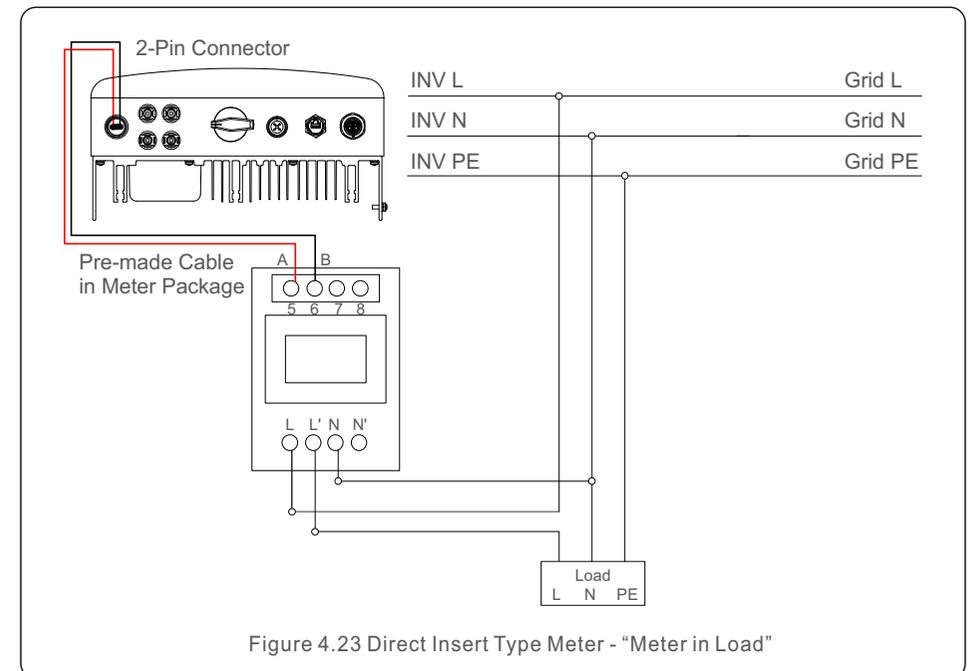
Figure 4.23 Direct Insert Type Meter - "Meter in Load"
