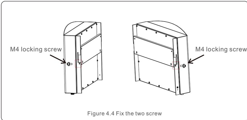
Figure 4.4 Fix the two screw
