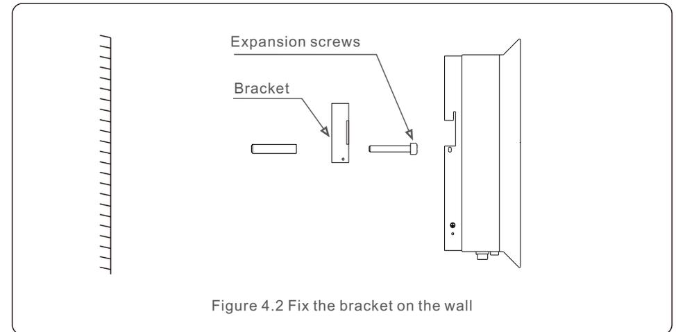
Figure 4.2 Fix the bracket on the wall
