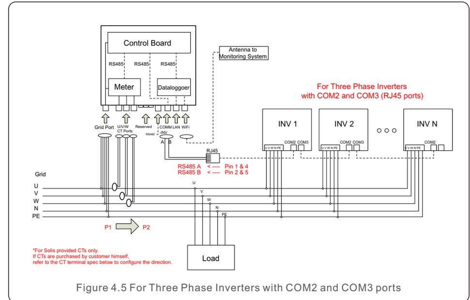
Figure 4.5 For Three Phase Inverters with COM2 and COM3 ports
