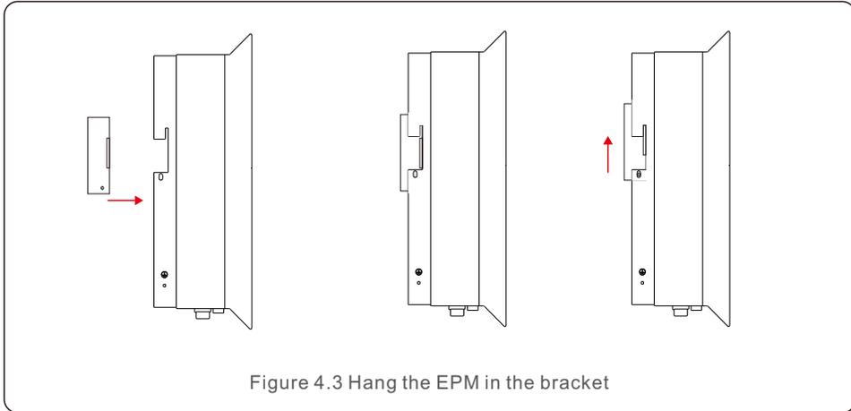
Figure 4.3 Hang the EPM in the bracket
