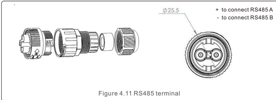
b. Refer to figure 4.11, connect communication cable between inverter with EPM, and then measure the distance from EPM to inverter. Use proper cable for RS485 connection. (0.5mm<sup>2</sup>)
