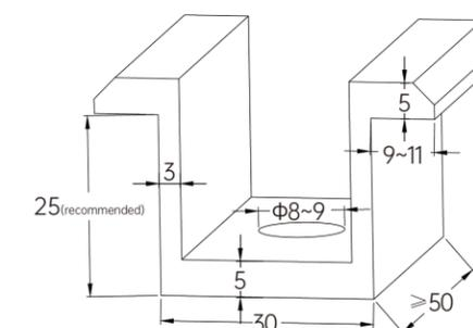
Under no circumstances should the clamp touch the glass or deform the frame. Be sure to avoid shadowing effect from the pressure clamp.
