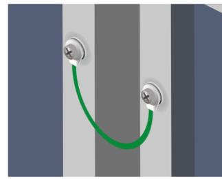
We recommend using the following method to ground correctly, as shown in the figure.
