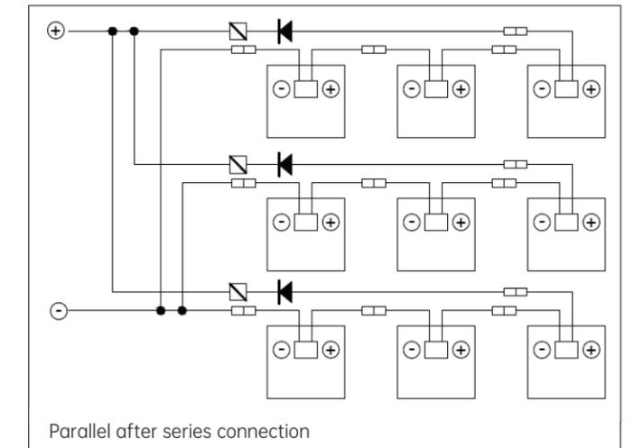
If there has reverse current exceeding the maximum fuse current flowing through the module, use overcurrent protection device with the same specifications to protect the module. If more than two strings are connected in parallel, there must be an overcurrent protection device on each strings of module.
